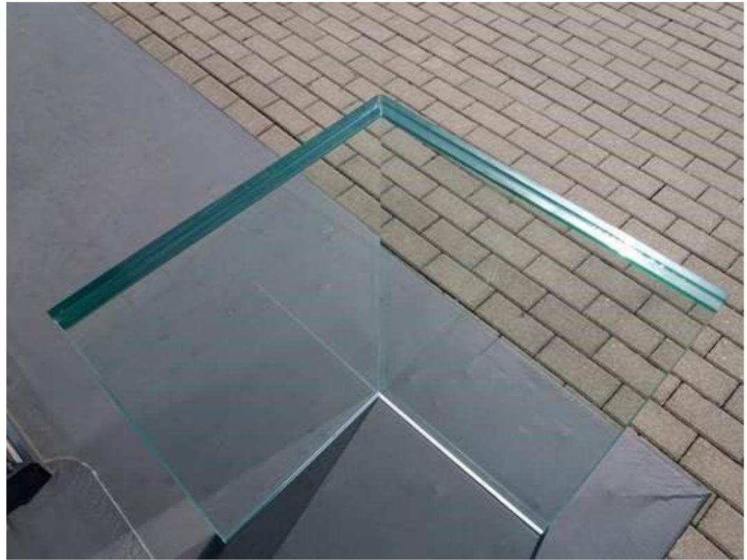
Two glasses which are laminated in 90 degrees without any bonding materials such as UV glue or silicon. It is purely made by lamination.
